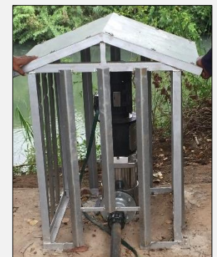
Solar pump powering smallholder irrigation
